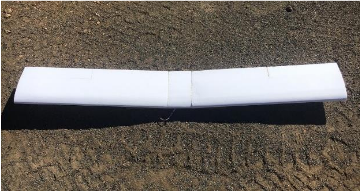
Figure 1 - Airplane wing with dihedral
