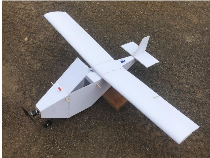
Figure 2 - Cargo hold access and dowels used to secure wings
